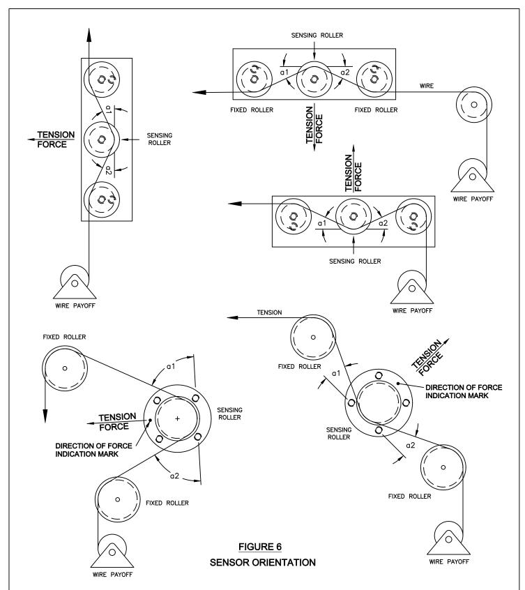
The tension sensor may be mounted in any position or orientation as long as the direction of force is maintained as shown above. The angles of deflection (a1 and a2) should be approximately equal, referenced to the sensors direction of force.
